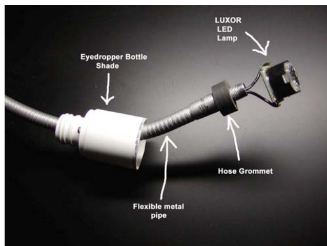
Figure 4. Lamp attachment to flex pipe with shade
