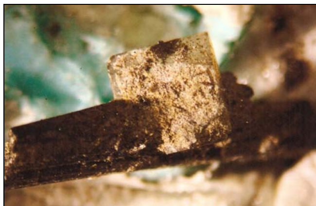
Figure 1b Showing the specimen after a one hour run in a detergent only solution
