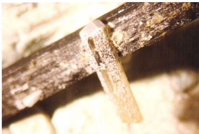
Figure 3 Natrolite on Aegerine with epitactic Tetranatrolite after a run in Super Iron Out, but not in the oxalic acid solution
