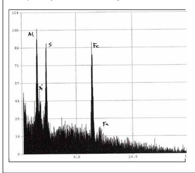
The EDS spectrum, to the left, for the white, crusty mineral indicated an Iron Aluminum Sulfur species.
