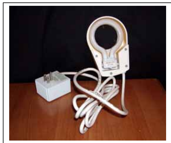
Figure 4: A repaired commercial fluorescent ring bulb illuminator salvaged from the trash.
