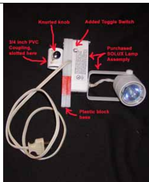
Figure 5: SOLUX lamp fixture adapter.
