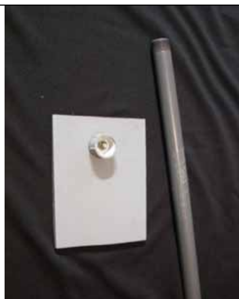
Figure 6: Lamp base assembly, steel plate with PVC end cap bolted on. Mouse mat cemented to backside. Pipe detached for view.
