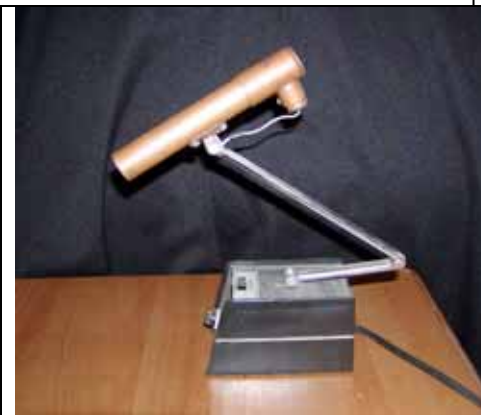
Figure 3: My first home-built microscope illuminator.
