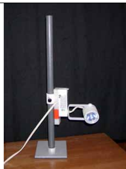
Figure 7: Completed SOLUX microscope illuminator
