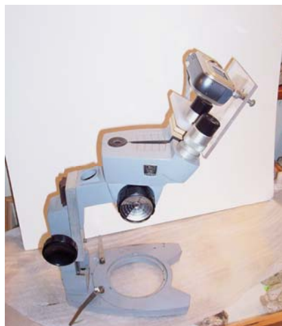
Figure 2: Adapter, digital camera, and microscope.
