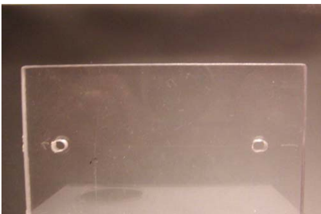
Figure 7: Elongated holes in Plexi piece for “x” axis adjustment.
