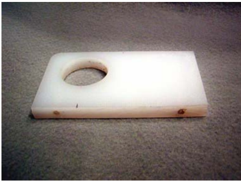
Figure 3: Nylon press-fit microscope attachment piece, (approx 4" x 2 1/2").
