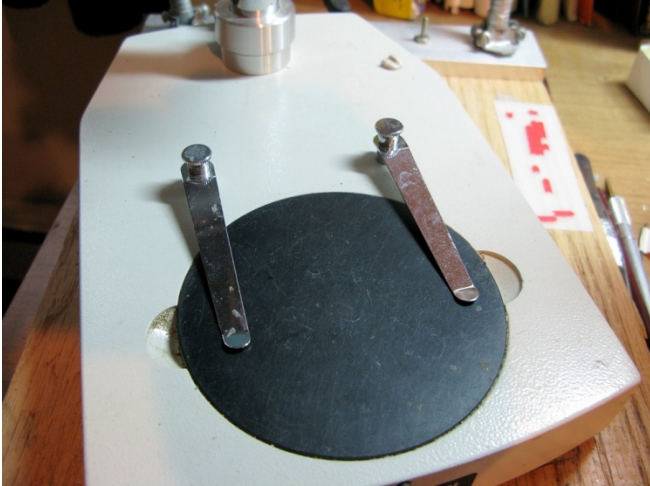
Figure 2: Slide holder clamps – typical of many stereo scopes.
